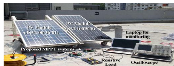
Fig. 12. Test setup for distributed MPPT.
