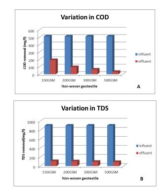
Fig 4.3(A) and (B): Graph showing the variation in COD and TDS after filtering through nonwoven geotextile
