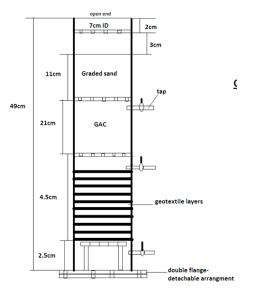
Fig 1.1: Schematic representation of column setup
