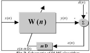
Fig-2: Schematic of DLMS algorithm
