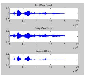
Fig-6: Result of LMS adaptive filter
