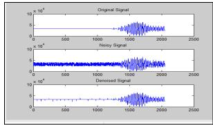
Fig-9: Result of RDLMS Adaptive filter
