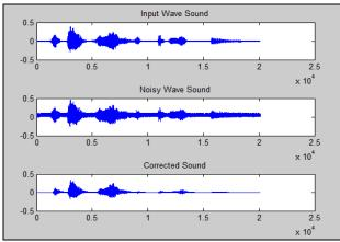
Fig-8: Output of DLMS Adaptive filter in MATLAB
