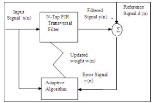
Fig-1: Schematic of LMS algorithm
