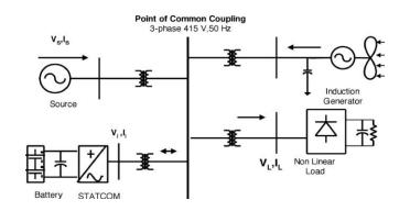
Fig.9.Grid Connected System for Power Quality Improvement
