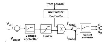
Fig.6 Control Scheme of STATCOM
