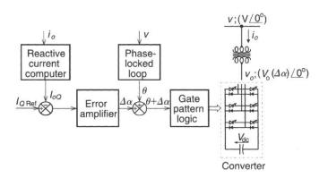
Fig.7. Main Function of the Internal Converter Control
