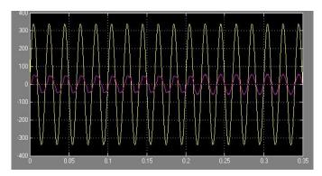
Fig.16.Supply Voltage and Current at PCC
