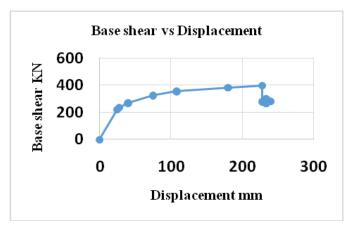
**Chart-1:** Base shear v/s Displacement curve for bare frame structure
