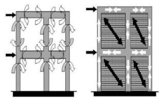
Fig-4: Behaviour of bare frame and infill frame under lateral load
