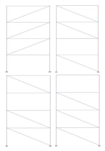
**Fig-3**: Elevation of infill frame with soft storey at different floor.
