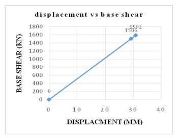
**Chart-2**: Base shear v/s displacement curve for infill frame structure
