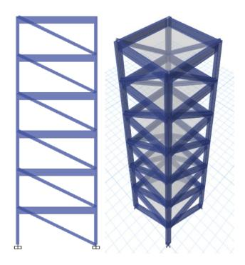
Fig-2: Elevation and 3D view of the infill frame model
