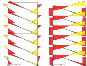
Fig-6: Bending moment and shear force diagram
