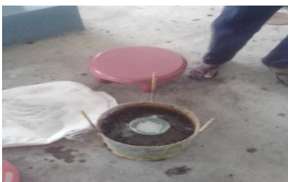
Figure : Filling the sand column materials
