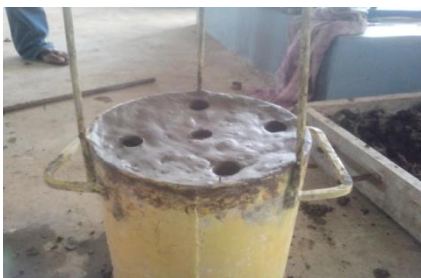
Figure : Group of columns in mould
