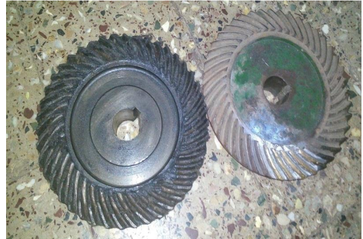
Fig.No.2.The image of Failure of face gear
