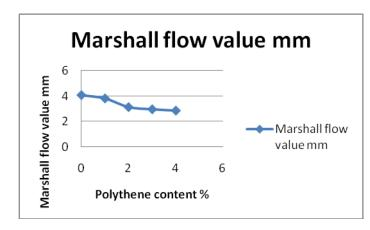
Figure-3: Marshall flow value vs. Polythene content
