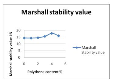
Figure-2: Marshall Stability value vs. Polythene content
