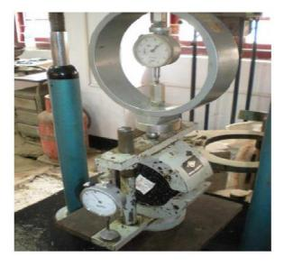
Figure-1: Marshall Test in progress
