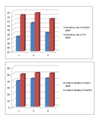
From the above graph the normal cube result increased for GFRP wrapping by 8.10%. and for hybrid concrete by 8.9Mpa when compared to without gfrp
