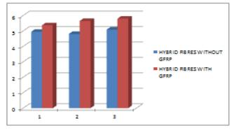
From the above graph the normal mix with gfrp have increased by 4.61% and for fibre added concrete by 12% when compared to without gfrp
