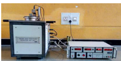
Fig-2. Schematic of Pin-on-disc wear test machine
