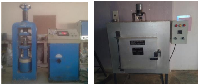
(a) (b) Fig-1: Equipments (a) Compression testing machine (b) Sintering furnace
