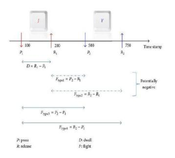
Fig -2: Flight and Dwell Time Measurement.
