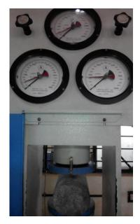
Fig -2: Split tensile test setup
