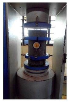
Fig -4: Modulus of elasticity test setup
