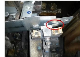
Uneven contact gaps between side member upper outer and the deformation element bracket
