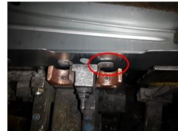
Uneven contact gaps between side member upper outer and the deformation element bracket
