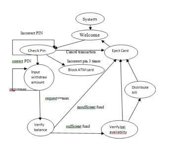
Figure 4:- Data Flow Diagram of Existing Working Of ATM System
