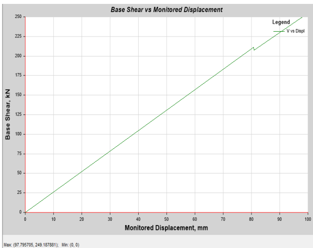
Fig 5.7: Pushover Curve with outrigger at 5 th storey
