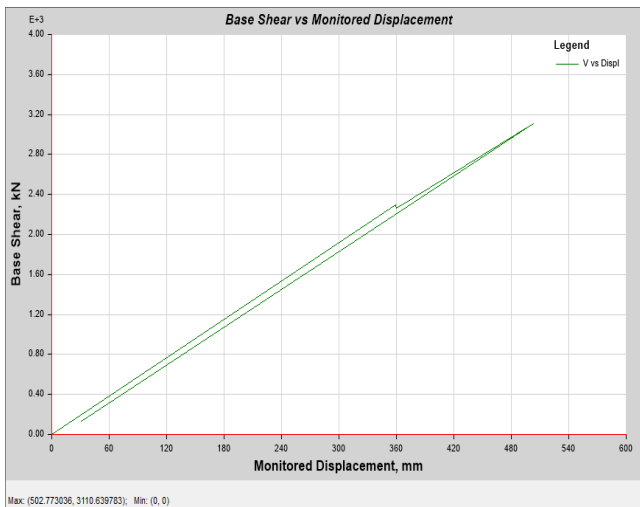
Fig 5.6: Pushover Curve without outrigger
