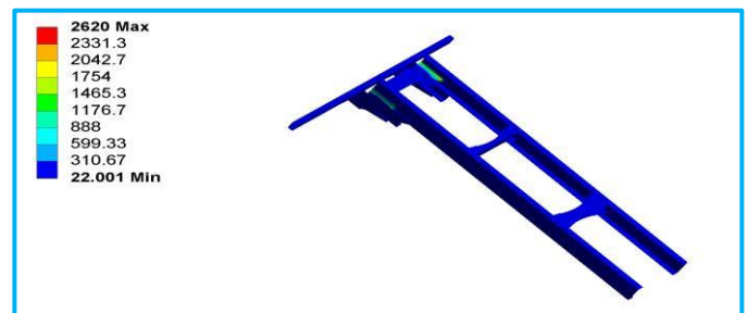
Figure-4 Temperature output for first four plates in Transient thermal analysis is 2620°C.
