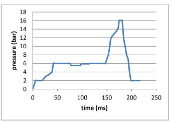
Fig-12 system pressure behavior while bending copper alloy 3 mm thickness
