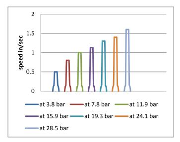
Fig -9 linear speed of hydraulic cylinder with 30% command value
