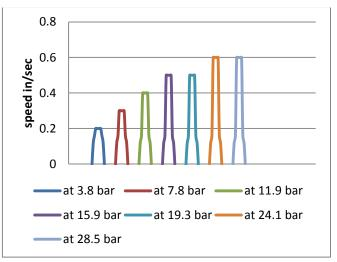
Fig -8 linear speed of hydraulic cylinder with 20% command value
