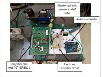
Fig -3: The Electro-hydraulic system
