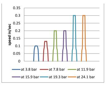
Fig -7 linear speed of hydraulic cylinder with 10% command value
