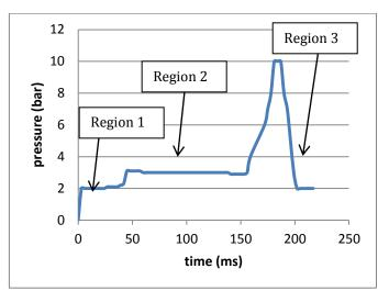
Fig-11 system pressure behavior while bending copper alloy 2 mm thickness
