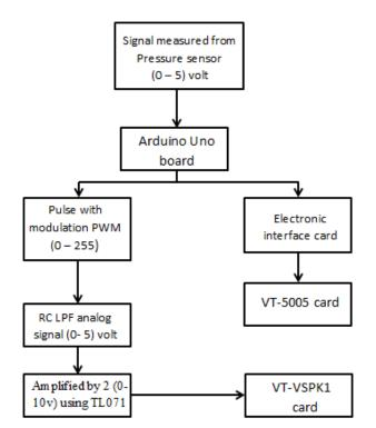
Fig -4: Block diagram of electronic circuit
