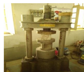
Fig:2 Testing of cubes under UTM machine
