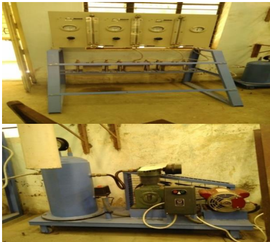
Fig 3: permeability test set up
