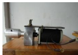
Fig 8 motor with aluminum hub
