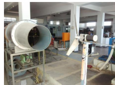
Fig 11 wind tunnel with wind turbine made of aluminum blades
