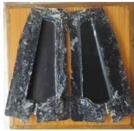
Fig 5 Patterns made for fiber Blades
