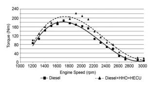
Fig -3: Variation of engine torque with engine speed [9].
