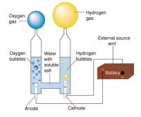
Fig -5: Experimental setup of electrolysis of water [12]
