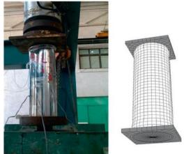
(a) (b) Comparison of deformed shapes at failure for circular hollow section specimen (a) Experimental and (b) Numerical
