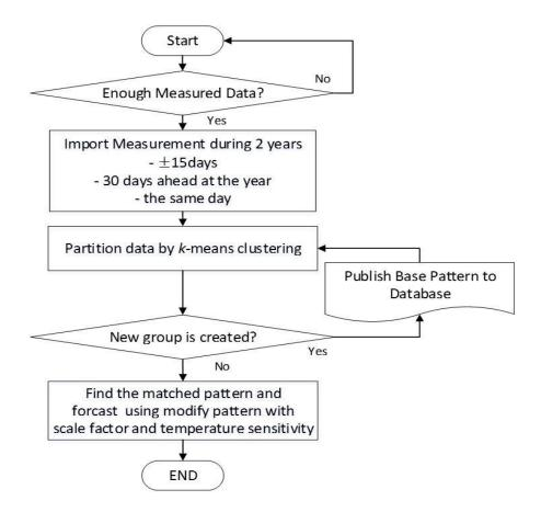
Fig. 2. Flowchart of the VSTLF for the electrical and heat load.
