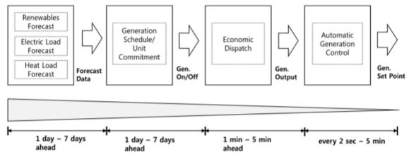
Fig. 1. Process flow of the generation applications package
