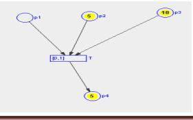
At the 5<sup>th</sup> iteration the process is stopped, since there are no enough tokens available in p1 to process and so the expected result was not derived. This is one of the limitations in Queuing Petri net.
