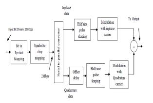
Fig 1.1 Block Diagram of ZigBee
