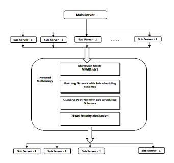
The multi mechanism hybrid model is shown in figure 1.2 . The high capacity main server serves the entire client's needs and requests. Different application uses
