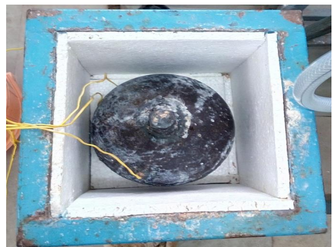
Fig6: storage tank with spherical ball
