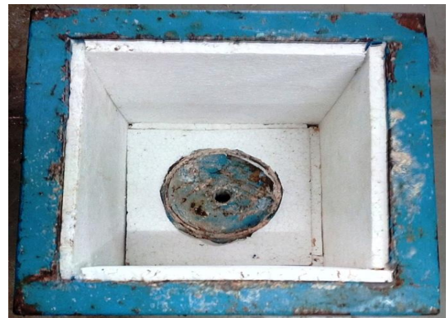
Fig5: Insulated with thermocole
