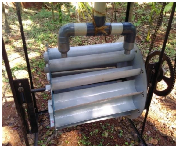
Fig.5: Second phase turbine diagram using T- shape reducers
