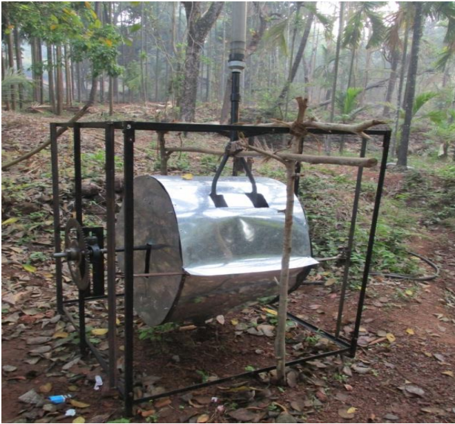
Fig-3: Complete developed pico hydro power generation model with casing of turbine
