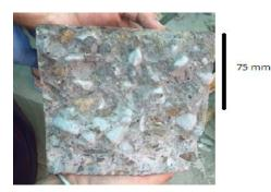
The concrete cubes coated with Type C coating were further subjected to a pressure of 10 kg/cm<sup>2</sup> for 48 hours. The average water penetration depth through the concrete cubes was observed as 150 mm
