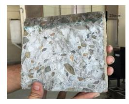
The pressure of the apparatus was further increased to 10 kg/cm<sup>2</sup> with regular increment of pressure from 5 kg/cm<sup>2</sup>. The average water penetration depth through concrete cubes after a period of 24 hours was observed as 80 mm.
