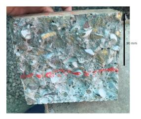
The pressure was again increased to 5 kg/cm<sup>2</sup> with subsequent increments in pressure. The average water permeability through concrete cubes was observed as 150 mm.
