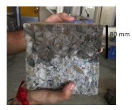
The concrete cubes coated with Type A were further subjected to a pressure of 10 kg/cm<sup>2</sup> for 48 hours. The average water penetration depth through the concrete cubes was observed as 150 mm.
