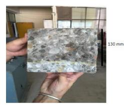
The pressure was further increased to  $5 \text{ kg/cm}^2$  for a period of 24 hours and the water penetration depth was recorded as 150mm.
