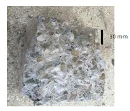
The Type C sample was subjected to pressure upto 10 kg/cm<sup>2</sup> and the average water penetration depth was recorded as 75mm.
