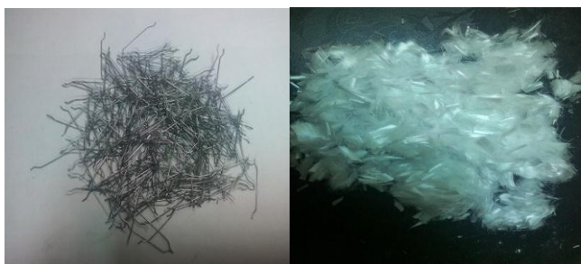
Fig -1: Steel and Polypropylene Fiber
