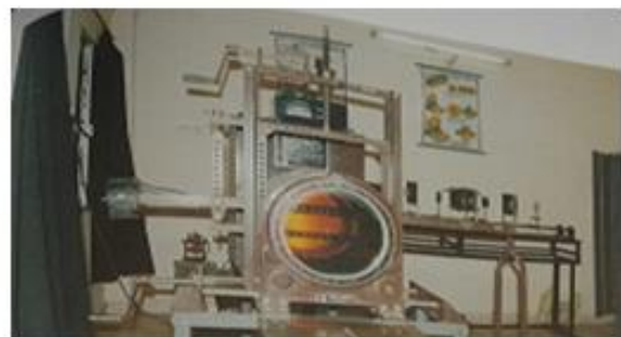
Photograph A- Polariscopes
