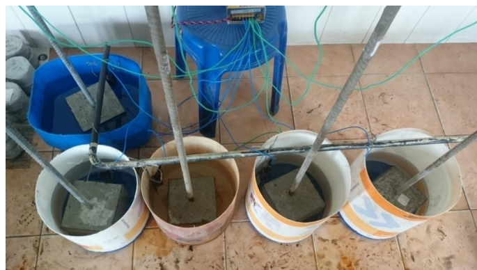
Fig.1 Accelerated Corrosion Setup
