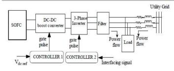
Fig. 2. Schematic diagram of grid connected DGs
