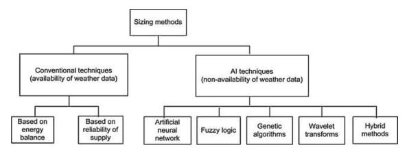
Figure 2 Classification of hybrid system sizing methods
