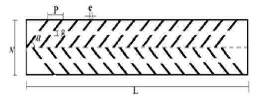
Fig 2 :- Schematic diagram of double incline ribs with gap
