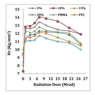
Fig 1: Variation of  $H_v$  with various doses of gamma irradiation at 60 g specimen of PVC, PMMA and PVC:PMMA with different wt% of PMMA.
