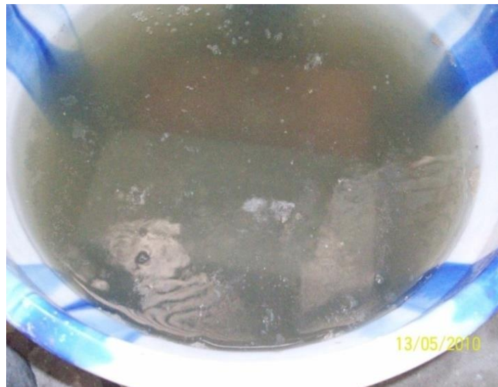
Fig.6 Different types of Bricks immersed in acids
