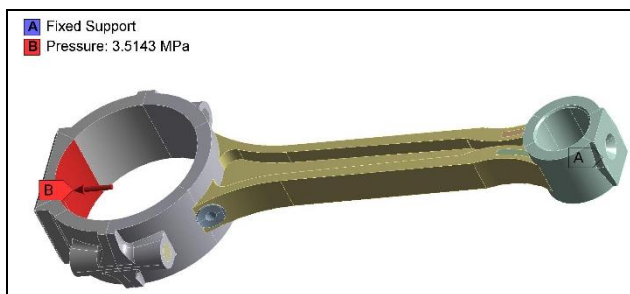
Fig -2: Boundary conditions of Connecting Rod with titanium inserts
