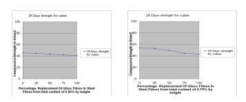
Graph -3: 0.5% & 0.7% of Replacemnt of Glass Fibers in Steel by weight for cube.
