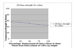
**Graph -4**: 1.00% of Replacemnt of Glass Fibers in Steel by weight for cube.
