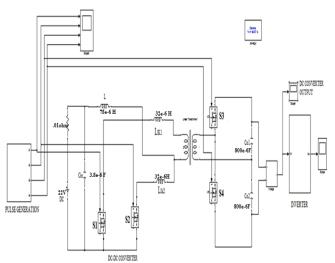
Fig -10: Simulink Model of Proposed System
