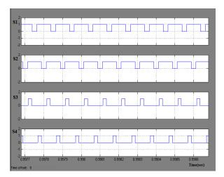
Fig -11: Switching Pulses of dc-dc Converter
