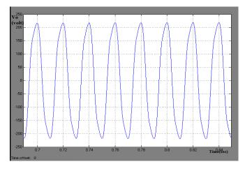
Fig -13: Full Bridge output for 12V input
