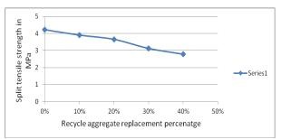
**Chart-2:** Recycle aggregate replacement Vs Split tensile strength for 28 days
