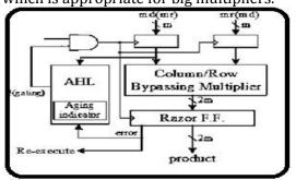
Fig.1. Block diagram of Proposed System II. IMPLEMENTATION
