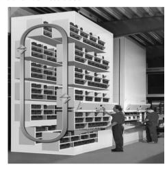
Fig.1.Vertical Carousel Storage System used in industry  $_{\left[ 1\right] }$
