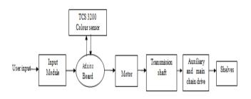
Fig.5 The block diagram for working system
