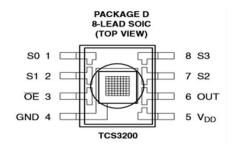
Fig.3. Pin Diagram of TCS 3200 sensor
