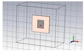
Figure 2: A Rectangular microstrip patch antenna without slots
