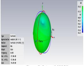
Figure 7: Gain at 0.932GHz
