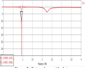
Figure 5 : Return Loss with slots
