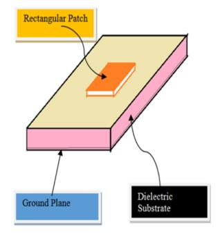
Figure 1: A Basic Rectangular Microstrip Patch antenna
