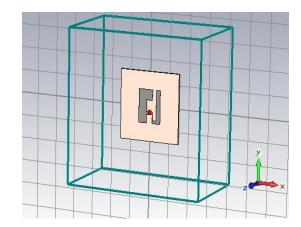
Figure 3: A Rectangular Microstrip Patch Antenna with slots
