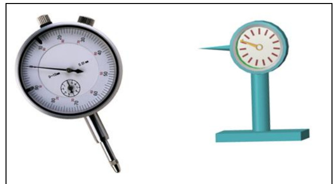
Fig.-20: Dial gauge indicator and its 3D model
