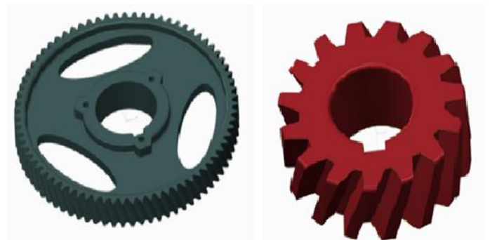
Fig- 17: (e) 75 teeth gear. (f) 16 teeth Pinion
