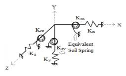
Fig-3: Equivalent spring stiffness.
