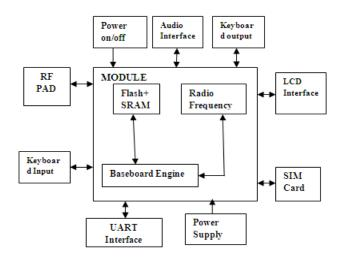
Fig.II: GSM module structure
