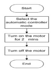
Fig.V.Flow chart of Automatic Mode
