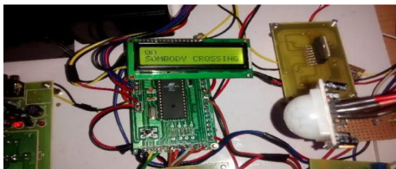
Fig-2: Human Detection Using PIR Sensor
