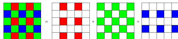
Fig.2: Bayer pattern used in single-chip digital cameras
