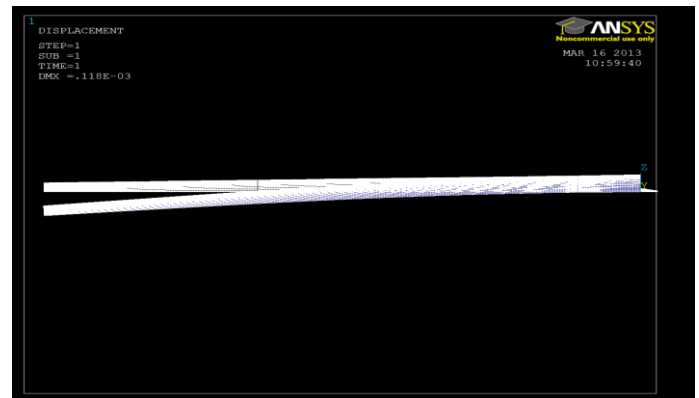
Fig-e: deformed+undeformed shape for carbon epoxy
