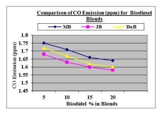
Chart-7: Comparison of CO Emission (ppm) for Biodiesel Blends
