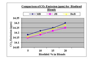
Chart-6: Comparison of CO<sub>2</sub> Emission (ppm) for Biodiesel Blends
