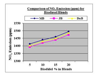
**Chart-8:** Comparison of NO<sub>x</sub> Emission (ppm) for Biodiesel Blends
