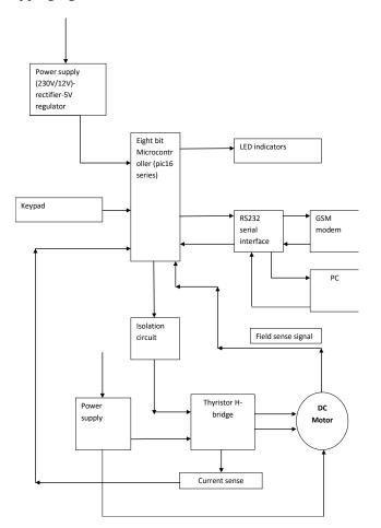
Fig.1 block diagram of the system
