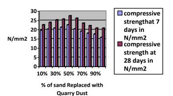
Figure : Compressive strength of 7, and 28 days for M20 grade up to 100% replacement of quarry dust.
